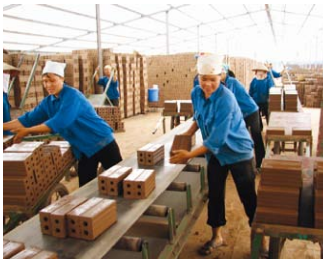
Over 300 VSBKs are already in operation in Vietnam where regulations also enforce better working conditions. Hollow bricks are popular.
