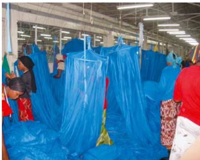
A to Z is a large textile mill in Arusha now producing long-lasting nets; the insecticide is already dissolved into the polyethylene granules
