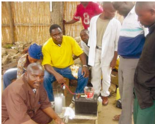
Antenna's small chlorine factory allows for decentralised production with simple means: electricity and cooking salt
